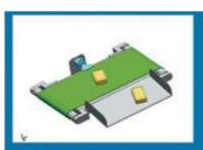
Air jet Suitable for small, thin products with light weight, or high-speed line.
