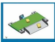
Air jet Suitable for small, thin products with light weight, or high-speed line.
