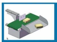
Pusher Suitable for small or large or thick packed products,
